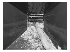
Hydraulic feed is standard on the Bobcat chipper.
