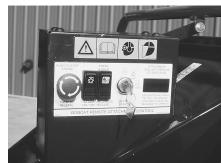
Using the Bobcat Remote Attachment Control Kit\*, the operator can start the loader from the ground without entering and exiting the loader. This eliminates the need for a second operator in the loader.
